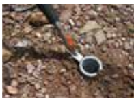
Setting pliers can be used to rotate trigger ring
