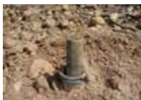
Wooden dowel prevents dirt filling CPE stake
